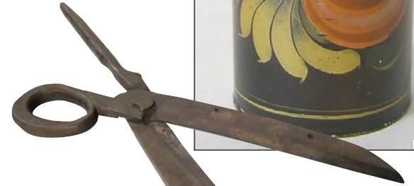
*Commonly used by both tinsmiths and at a printer's, these shears would be used by placing a stake through one of the handles and secured to the workbench in an upright position in a socket, allowing the tinsmith to operate the shears with one hand and allowing the free hand to turn the piece being cut. (photo: lancasteronline.com)*
