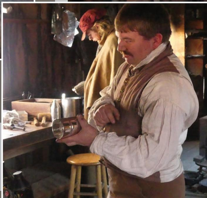
*At right: After soldering the joint of the cup, the tinplate worker shows off how smooth the soldered seam is. From here he can continue soldering the bottom and handle. Many items produced were round, as that is a very simple and easy shape to make quickly including cups, pans, coffee pots, and others.*
