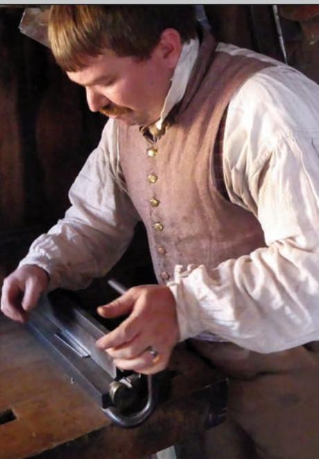
Far left: Making tin items often required forming a rolled edge. If the edge is straight, the tinplate worker uses a bar folder to fold the edge. Here a handle's edge is being folded 180 degrees over.
