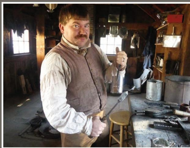
Here, the body of the cup was shaped and has been soldered to keep its shape and to make it watertight. The tool in his right hand is the soldering copper which has been heated in the charcoal fire to melt the solder.
