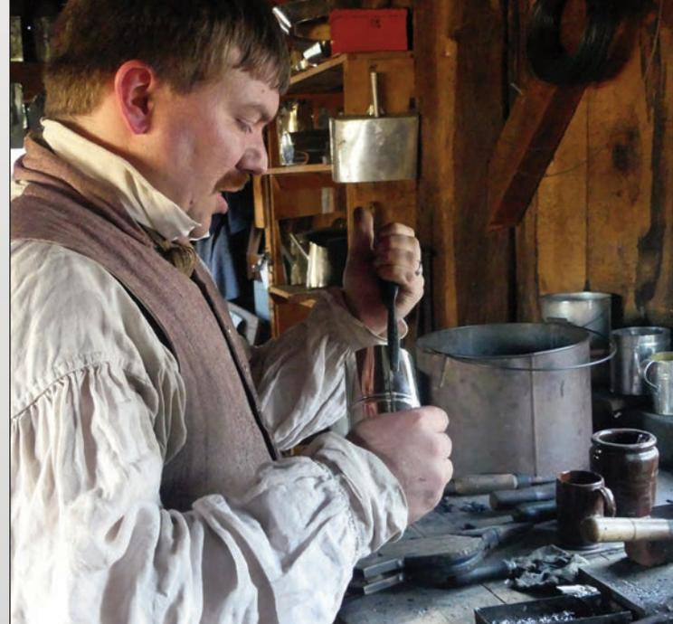
*After soldering the cups body, the solder hardens, holding the cup together and making that section water-tight.*
