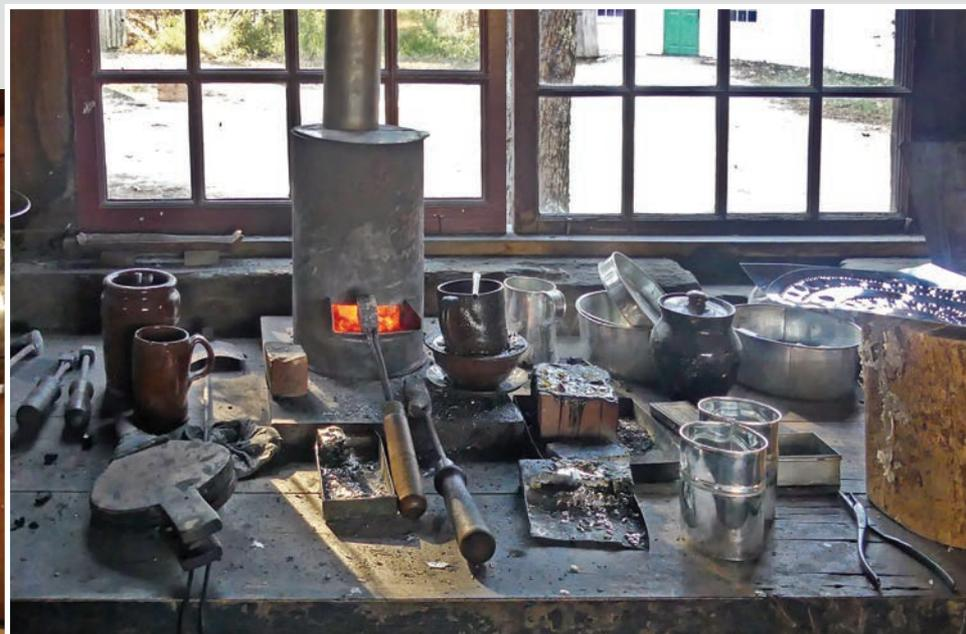
Take a look at the soldering stove. Prior to the 1850s the only fuel used was charcoal. Tin shops would make the stove themselves out of sheet iron. When using the tools to solder copper to tin, the tip of the tool would be placed in a fire hot enough to melt the solder.
