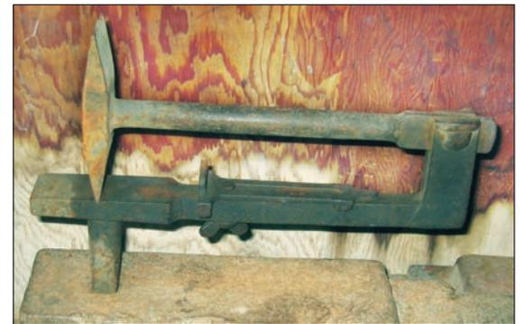
*This style of anvil was called a "stake" anvil and was used by the tinsmith to create creases in the metal for a variety of small items. This tool is seen placed on top of a blacksmith's anvil. (photo: ebay)*
